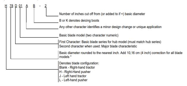
\*: Diameter limits are nominal diameters of the assembled propeller. They do not include the + or – 0,32 cm (1/8 inch) manufacturing tolerance the FAA allows for propeller with a basic diameter of less than 426,7 cm (14 feet).
